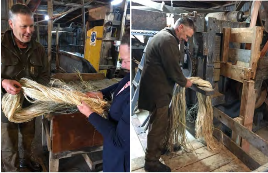
Vaughn (and Moira) checking the partially stripped fibre (above left); Vaughn feeding dry fibre into the next machine to remove further fibre (above right).
