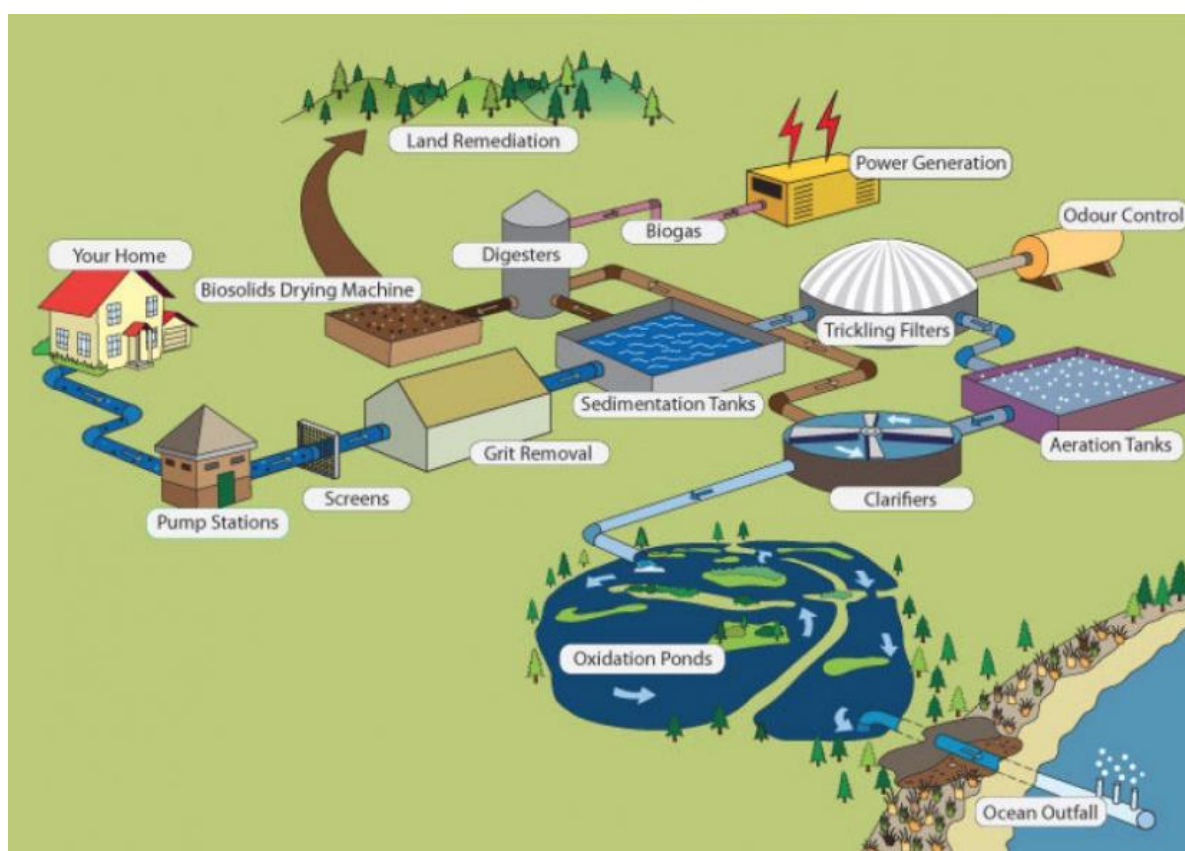
Figure 3.9: Typical wastewater system components (CCC, 2018)
