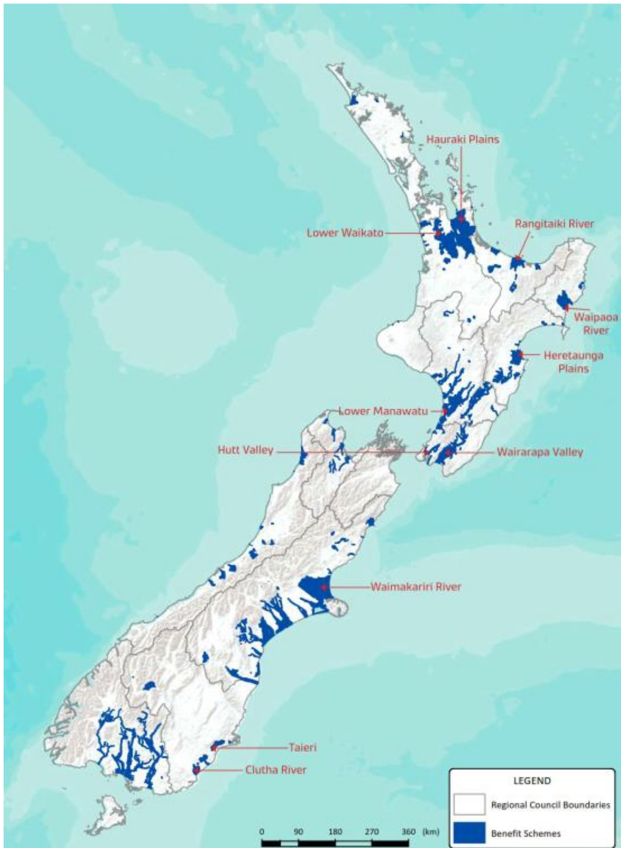
Figure 6.3: Extent of areas that receive a direct benefit from stopbank protection. Source: (T+T, 2018)
