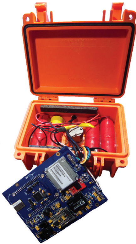
Fig. 1. The custom-made circuit board, lithium batteries and the watertight case.
