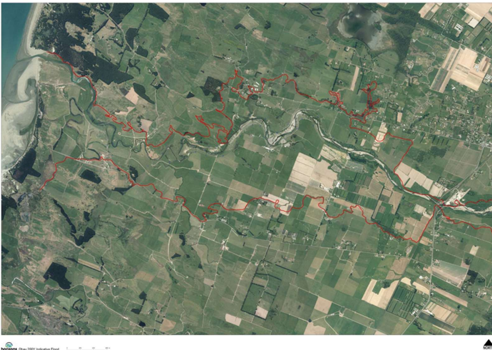
Figure 4.3.5 0.5% AEP (Annual Exceedance Probability) with 500mm freeboard "indicative floodable area" map. Ōhau River. Flow at ~700 m 3 /sec (Source: Horizons Regional Council).
